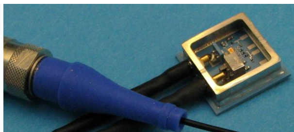
Fig. 2. VTT's SpaceFibre transceiver with LuxCis connectors before lid sealing.
